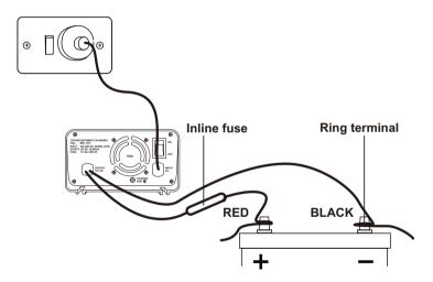
If the charger is used in a Permanent / Hard Wired application and the vehicle will not be used for some time, it is best to leave the charger connected to mains power (turned 'On') so that it can maintain the battery fully charged.
